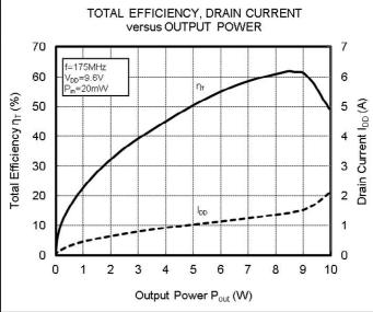
RoHS Compliance ,135-175MHz 8W 9.6V, 2 Stage Amp. For PORTABLE RADIO
