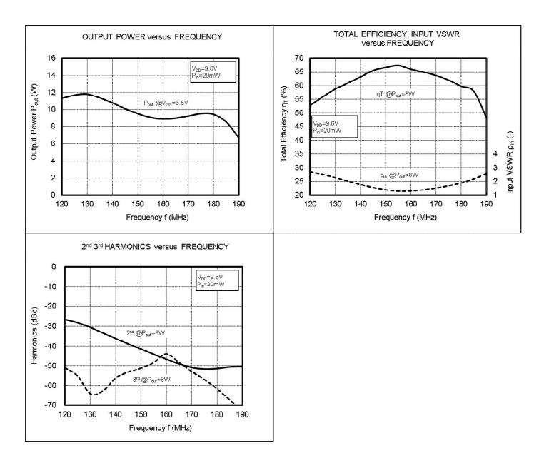
RoHS Compliance ,135-175MHz 8W 9.6V, 2 Stage Amp. For PORTABLE RADIO
