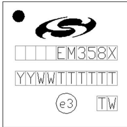
Figure 6.7. Part Marking for EM358x
